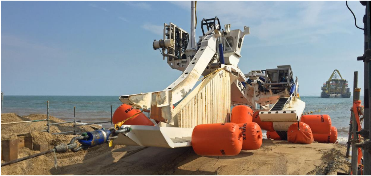
Figure 18: Boskalis' HD3 cable plough
