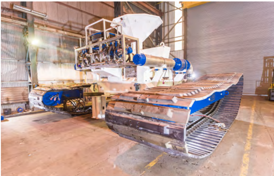
Figure 36: Jan de Nul's UTV1200 Mechanical cutter
